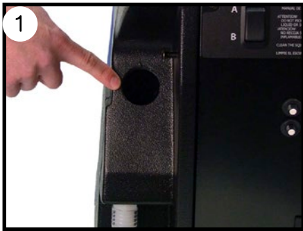
Rear hose fill port
