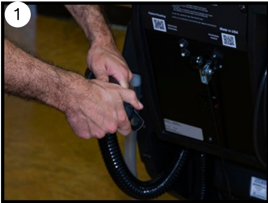
Check for clog in the restriction collar
