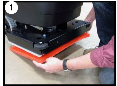
For pad removal on the orbital unit, simply pull off the pad
